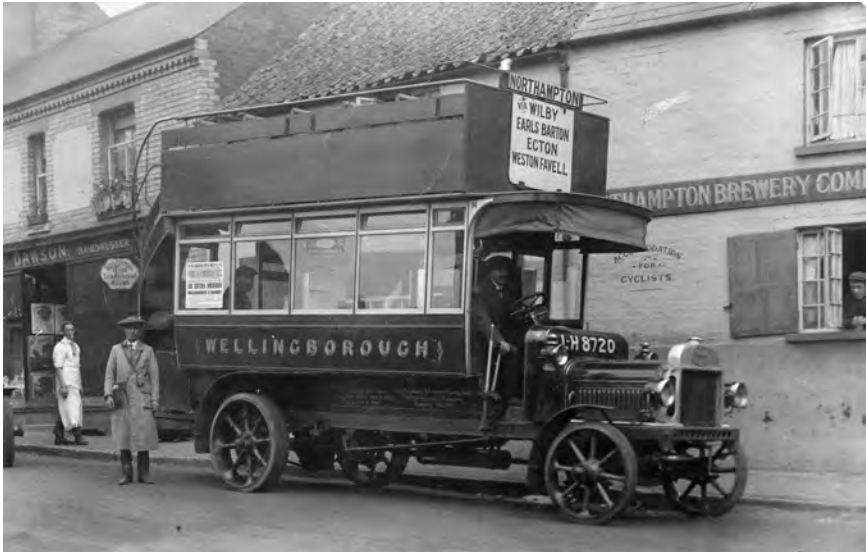
A 1914 Leyland ST of the Wellingborough Motor Omnibus Co Ltd standing outside the Bull Hotel, Irthlingborough in readiness for a journey to Northampton taking 1 hour and 25 minutes.
